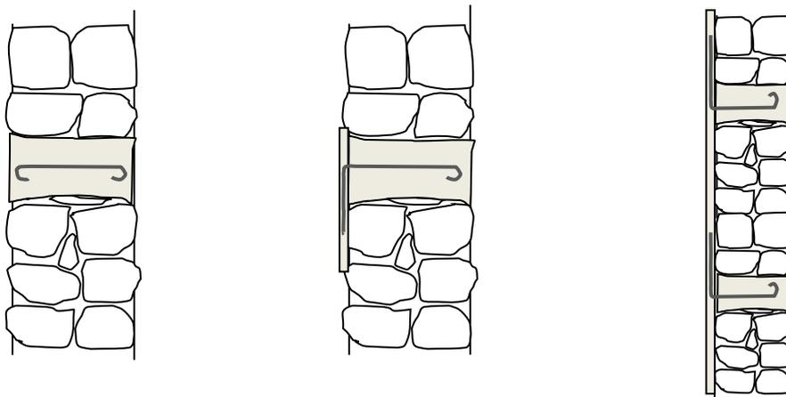
(a) Stitching element: stitches withes together. Length is 50mm shorter than wall width.
