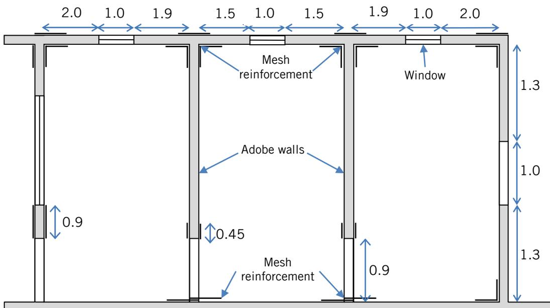
Figure 7: Illustration of wire mesh retrofit locations for a house in Guadalupe, Peru based on San Bartolome et al. (2004).
