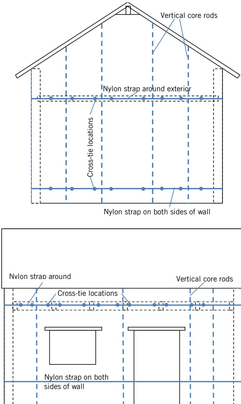
Figure 9: Sketch of vertical bar locations in experimental study by Tolles et al. (2000).
