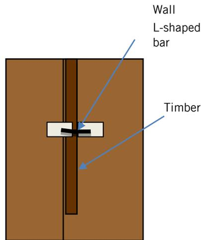
Figure 6: example improved connection between adjacent walls, based on UNDP India (2007).
