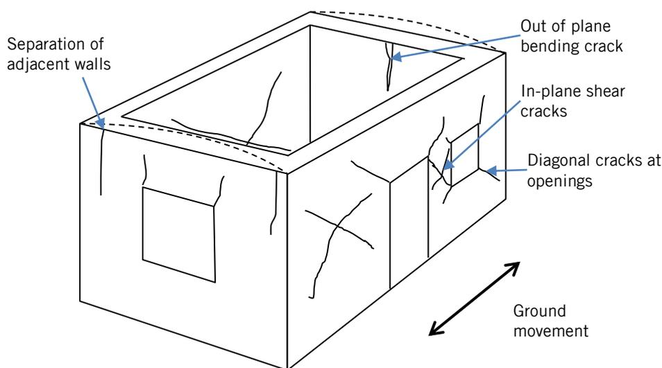
Figure 2: Damage typologies in unreinforced masonry.
